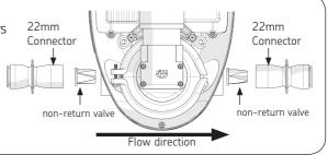
(8) Check that you have not overtightened and distorted the non-return valves before connecting the pipework. Refit the front cover.
