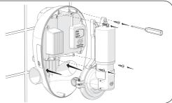
7 Fit the non-return valves as shown. Fit the pump connectors to the pump.
