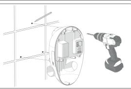
Mount the pump to the finished surface using all the wall fixings.
